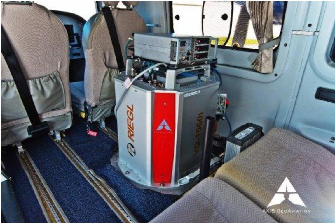
*One of AXIS GeoAviation's two new RIEGL VQ 1560i sensors, mounted in the Vulcan Air P68C*
