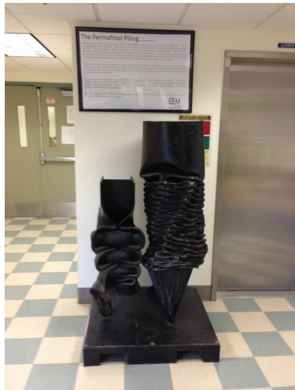
Photo: *H and Pipe Piles Meet Permafrost!* (From the lobby of the Geological Engineering Department, Uof A, Fairbanks)
