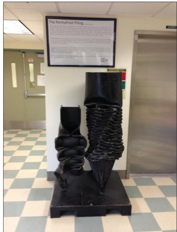
Photo: *H and Pipe Piles Meet Permafrost!* (From the lobby of the Geological Engineering Department, U of A, Fairbanks)
