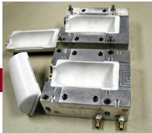
Figure 2: FDM hybrid tool with contoured insert mounted in a machined mold base
