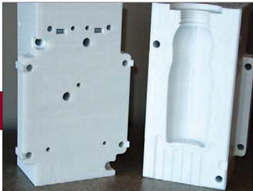
Polycarbonate (PC) blow mold made from the fused-deposition modeling (FDM) process
