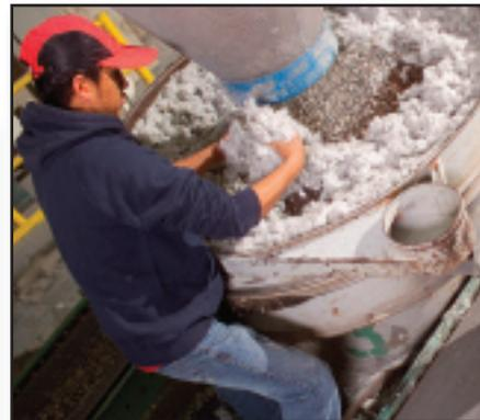
Nicos Polymers Group’s proprietary process for removing continuous-fiber reinforcement from flexible composites.
