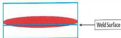
Figure 2: Ultrasonic Seal - An ultrasonic weld applies mechanical vibration between the sealing surfaces, creating frictional heat that melts the material on facing surfaces that are then compressed into a bond. Courtesy of Branson
