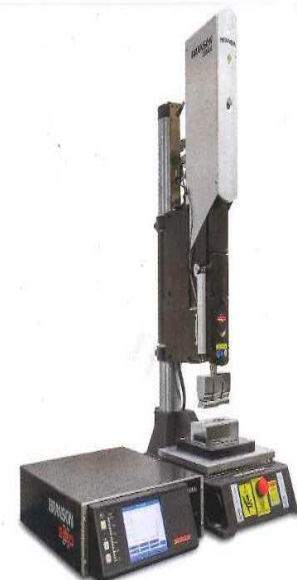
Figure 4: Ultrasonic welder, showing weld "stack"—An ultrasonic welder, like the Branson 2000 XC, includes a power supply (left), an actuator (top right, front) which contains a "stack" assembly consisting of a converter, booster and horn, and a base equipped with a metal fixture or "anvil." When production requirements dictate, modular versions of these ultrasonic welding components can be integrated into larger, automated assembly or packaging lines. Courtesy of Branson
